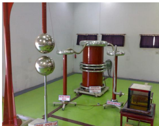
Fig.1. A photograph of the schematic experimental setup of partial discharge measurement
